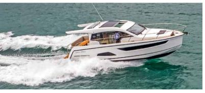
Sealine agent Windcraft has fitted a New Zealand-made stainless steel staple to the swim platform which supports the dinghy tender and outboard and also accepts a custom bait board for fishing. The fold-away swim ladder is stowed flat in the platform locker and drops into slots by the transom door on the starboard side when required and a pull-out freshwater shower washes the salt from swimmers' bodies.
