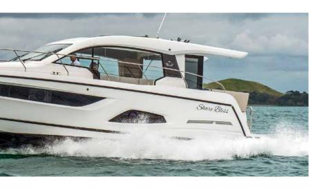
stern legs. This is the 'speed' power option, giving a top speed of 34 knots. The standard power option is a pair of four-cylinder D4 340hp engines good for 27 knots top speed.
